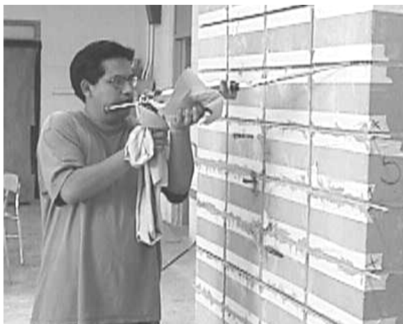
(a) Application of Embedding Paste
