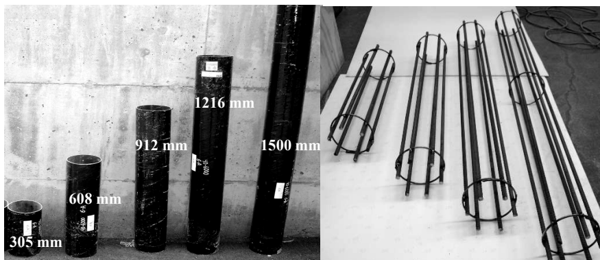
Figure 1. GFRP tubes and steel reinforcement preparation.
