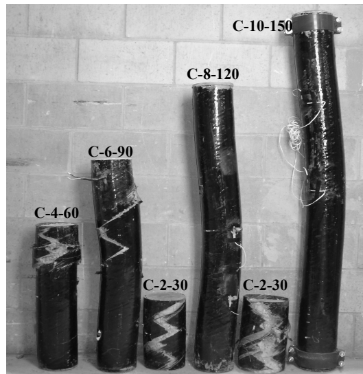
Figure 3. Different failure modes of the slender CFFT columns.
