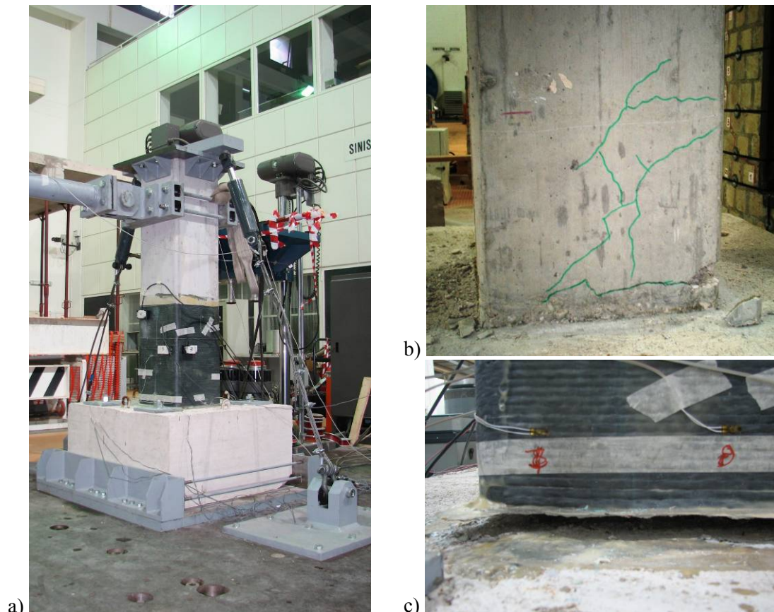
Figure 4. a) A40 test setup; b) A20 crack pattern at base; c) A20 crack opening at base;
