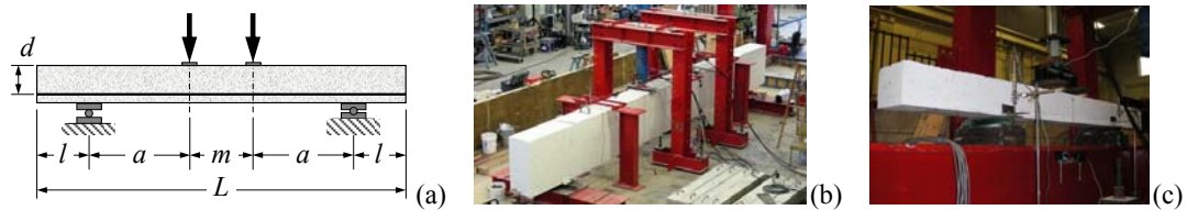
Figure 2. Test setup: schematic (a), and photograph of setup for Series S1 and S1B (b) and Series S6 (c).
