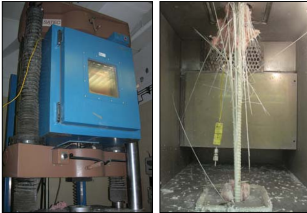
Figure 1. Setup for Cold Temperature Testing and Failed 16mm Test Specimen
