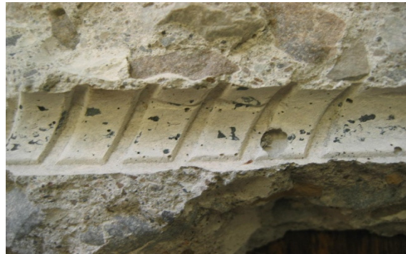
b) Failure plane for unwrapped beams (bottom cover)
