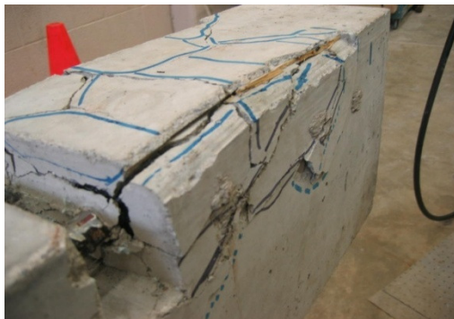
a) Concrete splitting
